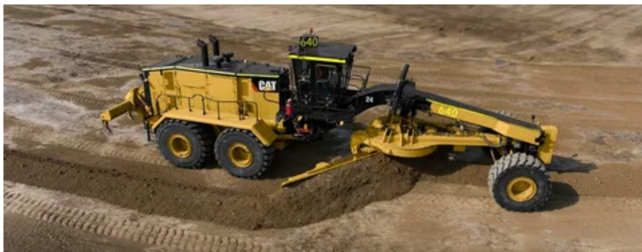
1-rasm. Caterpillar avtogreyderining gruntga ishlov berish jarayoni.
