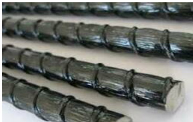
7-rasm. Mahalliy bazalt armaturalarining tashqi ko'rinishi
