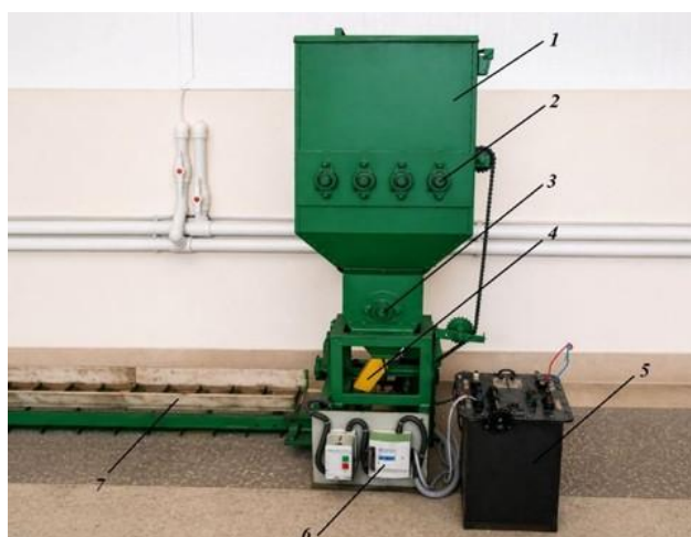
Figure 3. General view of an innovative seeder for sowing seeds of desert forage plants.
