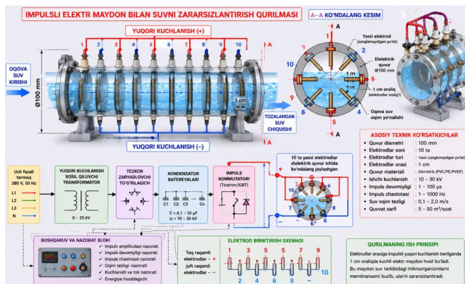
Figure 3. Wastewater disinfection device using pulsed electric field and its technological scheme
