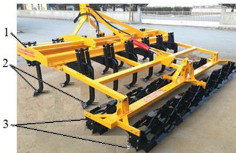
2-rasm. Turkiyaning “HELVACILAR” firmasining super og‘ir turdagi g‘altakmolali kultivatori
