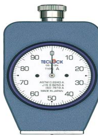
2-rasm. Rezinaning qattiqligini aniqlash jihozi GS-709N (Shore A)
