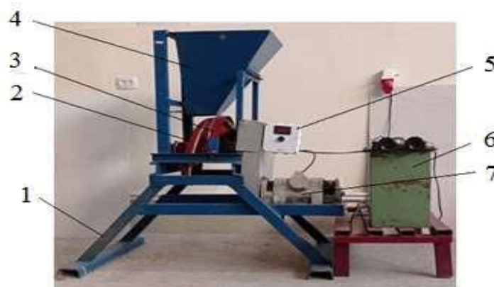
1-rama; 2-vintsimon pichoq; 3-quzg'almas pichog'i; 4-bunker; 5- tok va kuchlanish ulchagich; 6-latr; 7-elektrodvigatel
