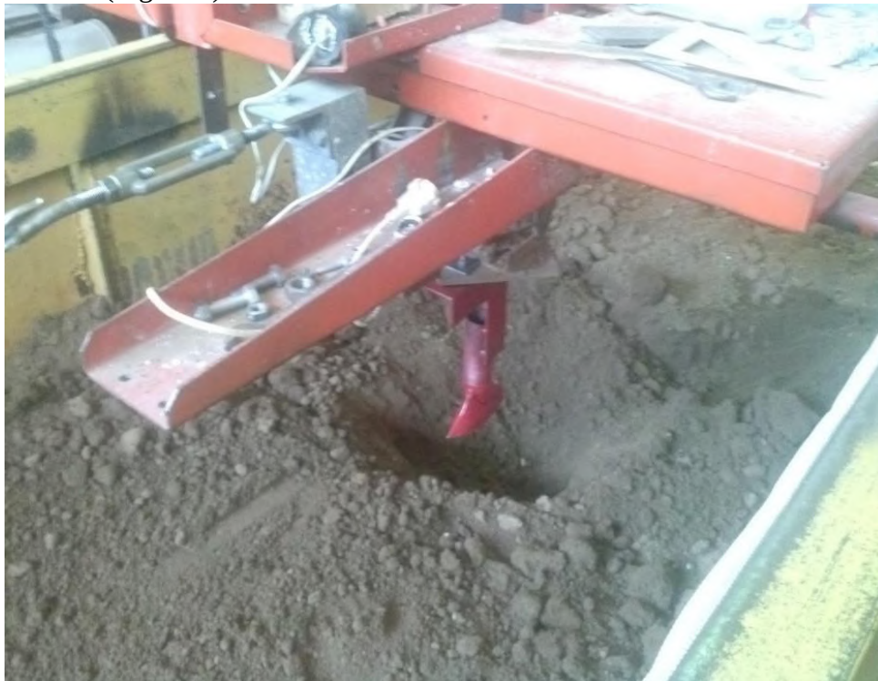
Figure 2. Testing the drip tape stacker model in the soil channel.
