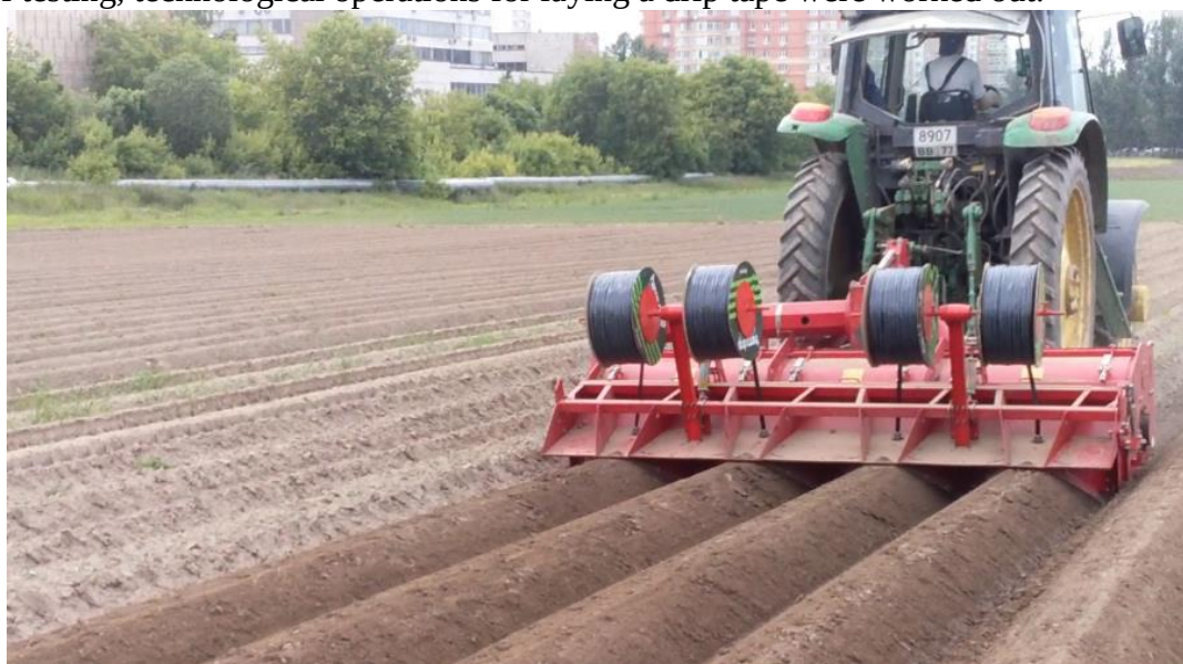
Figure 4. Laying drip tape while forming potato ridges.
