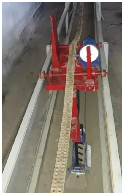
Figure 2. Side view of laboratory construction which creates a long pawl between cotton rows.
