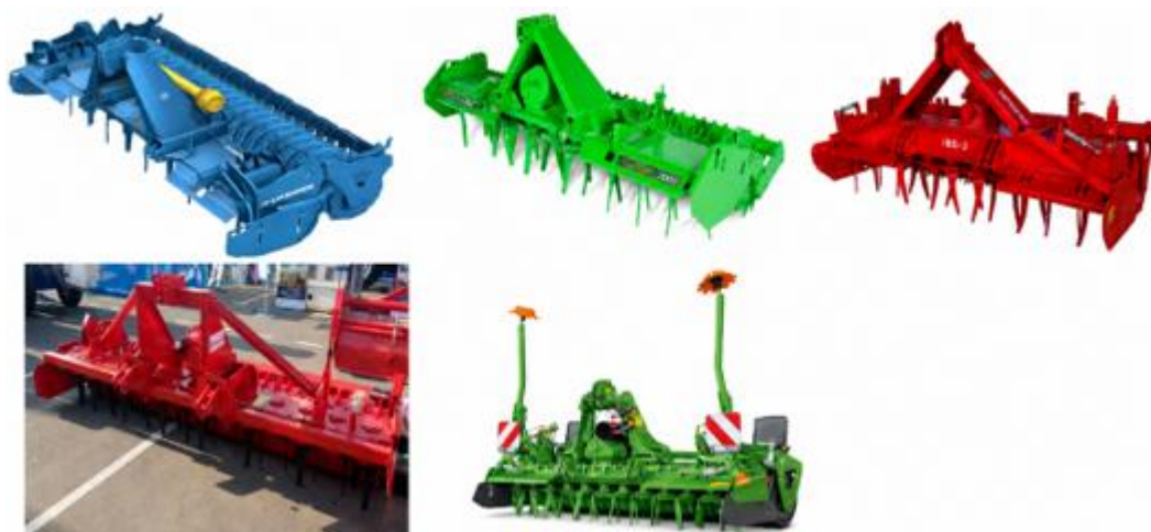
Figure 1. Existing vertical shaft rotary tillers used for pre-sowing soil preparation
