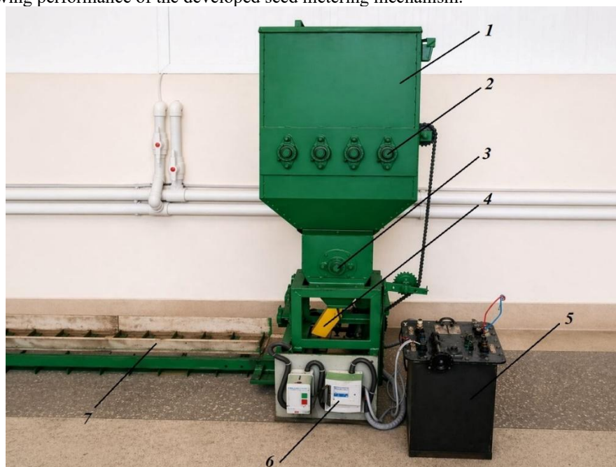
Figure 6. General view of the experimental machine prototype. 1-hopper; 2-shaft (on which a conical working element is mounted); 3-drum; 4-seed delivery tube; 5-variable transformer; 6-distribution panel; 7-belt conveyor
